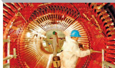
Stator repair on site
