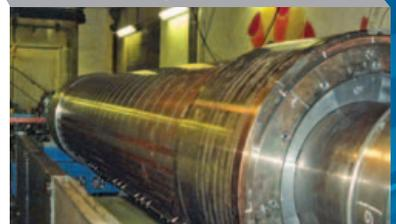
Rewinding 2 poles 250 MW rotor in factory
