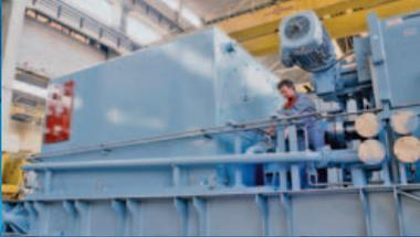
4 pole generator with flange mounted gear box
