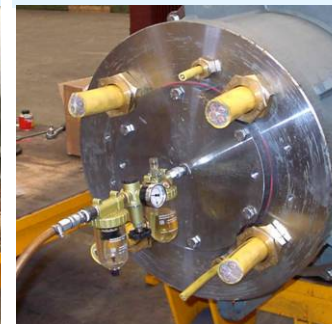
Seal-tight test with 2 bar
