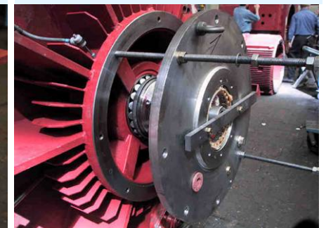
Assembly of the NDE cylindrical-roller thrust bearing
