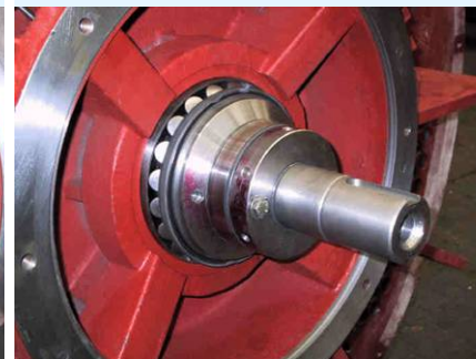
NDE with self-aligning roller thrust bearing
